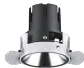
Model No.: P87 (Fixed Trimless) Product Size : ø85x95mm Cut-Out Size : ø90mm Optional Reflectors : White / Matt Silver / Chrome / Titanium Black
